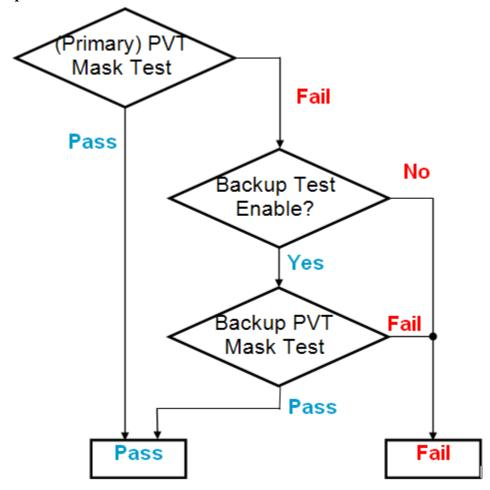
The PVT mask test is one of the most severe tests for GSM/EDGE. To reduce the total test time, in CGSM you can specify a set of backup bursts that are tested only when the primary bursts' mask test has failed. See the diagram above.
