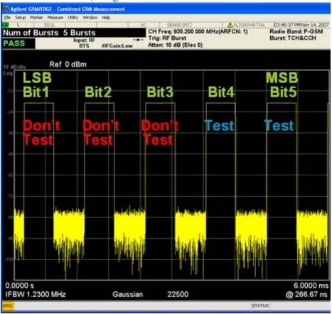
**Note**: the figure above is not an actual screen shot, but is used to illustrate how the Test Bitmap is used.
