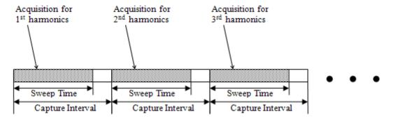
Sets the interval of capturing each harmonics. If the value is set to smaller than sweep time, it will be changed to the same value with sweep time.
