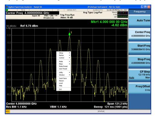
Placing the cursor on one of the menu rows marked with a right arrow symbol causes that row to expand, as shown in the example below, where the cursor is hovered over the "Utility" row:
