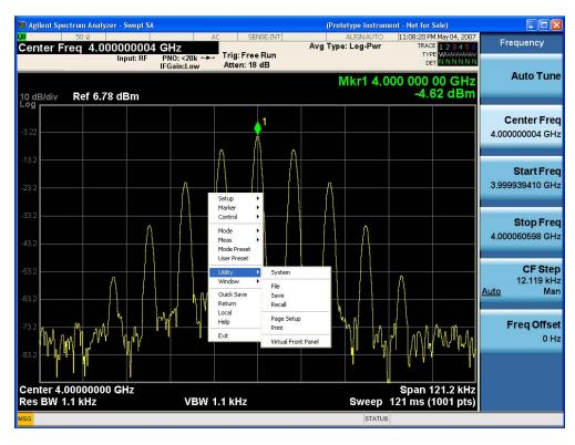
This method can be used to access any of the front-panel keys by using a mouse; as for example if you are accessing the instrument through Remote Desktop.
